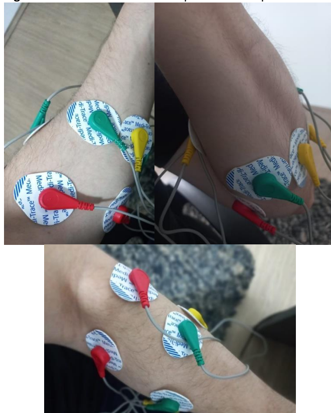
Figure 5. EMG sensor electrodes placed on the person's arm.
